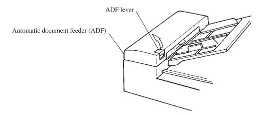
Figure 5.1 Removing jammed documents
